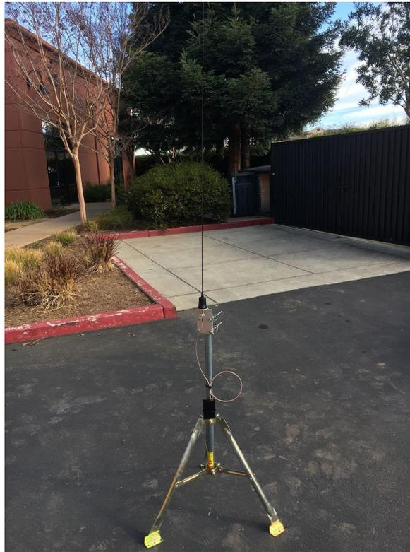
**Figure 4:** Example of mounting of Tracker with use of 1/2 Wave Antennas
