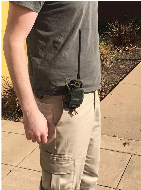
**Figure 5:** Example of body-mounted Tracker with Coiled 8.5" Antenna
